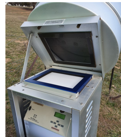
Air quality is currently monitored at McPhillamys by tools including (top) dust gauges and (bottom) a high volume air sampler.
