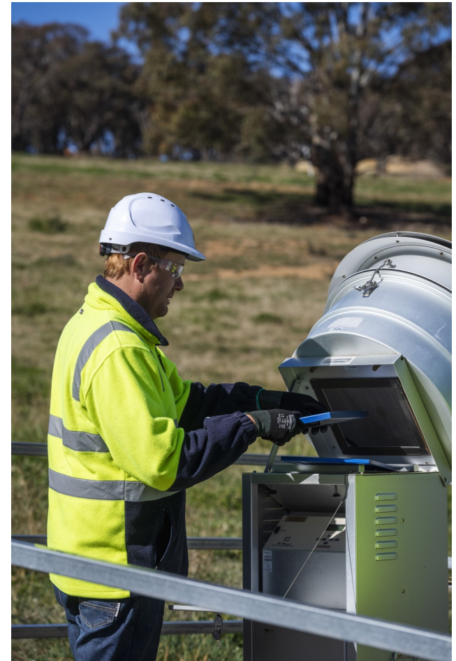
Above: Air quality and dust levels are measured by devices such as this High Volume Air Sampler on the McPhillamys Project site.
